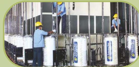
Fully automated temperature controlled PUF setup
